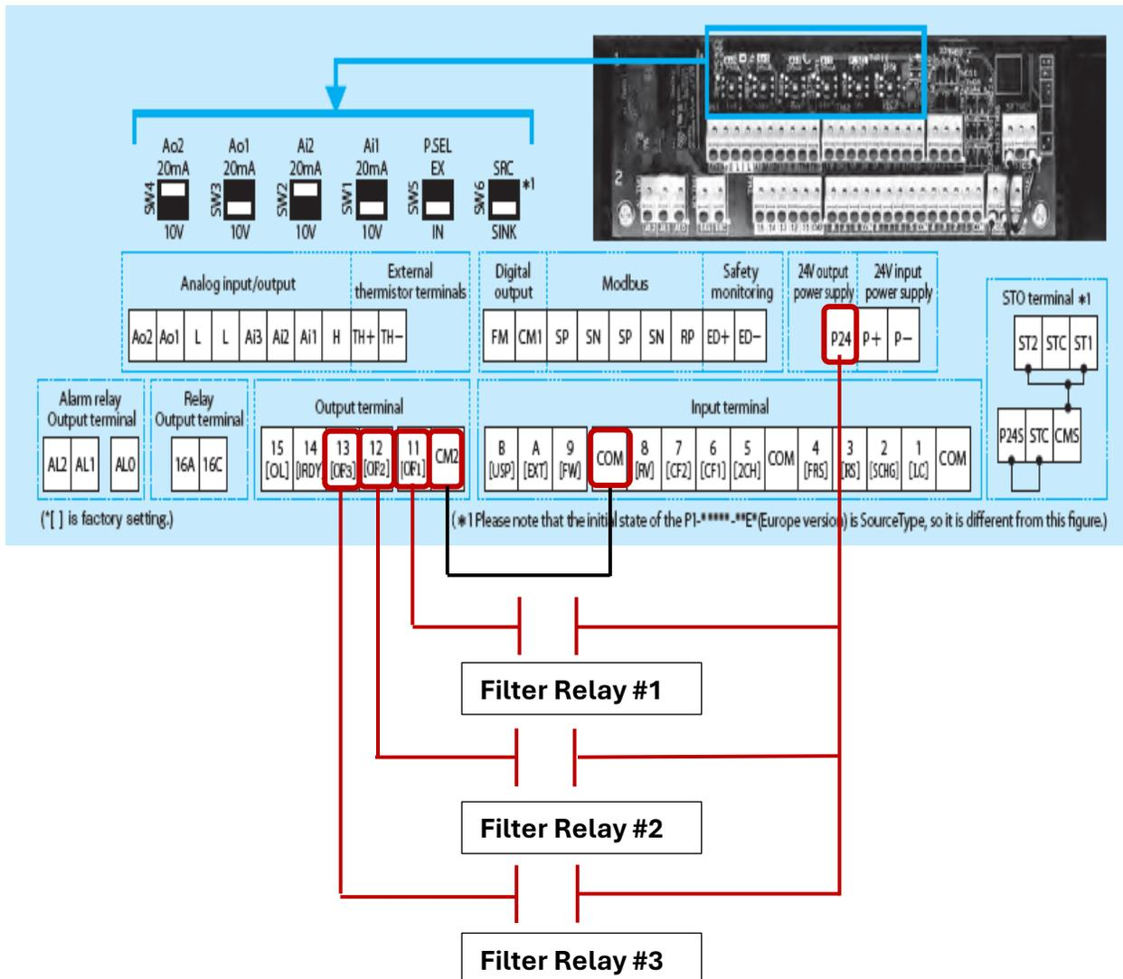
To activate the filter sequence function; first, set the “Number of Filters” field using the GUI webpage. Setting this field to 0 disables the filter sequence function. After setting the number of filters, please set the “Inlet Filter Times 1, 2, and 3” fields to the desired filtering time in seconds. Please see the Irrigation IOT User manual for more information on the filter function and the filter sequence function program flow diagram.
